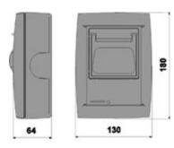
OBTPRB - Abmessungen in mm
